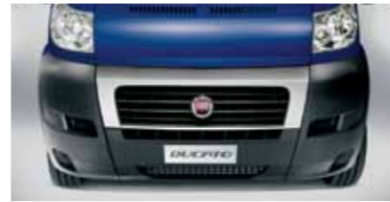
The front portion of the frame features a high-energy absorbing structure, and the front bumper of the Ducato comes in three separate segments making for lower repair costs in the event of a minor crash.
