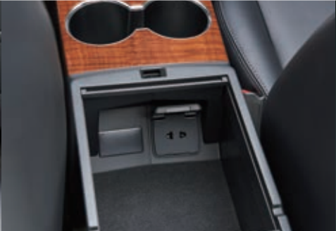
AC power outlet Simply plug in to power small electric devices up to 150W. Note: The maximum voltage and plug type may vary depending on market model.
