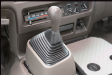
Fully synchronized manual transmission Short shift lever for easier shifting
