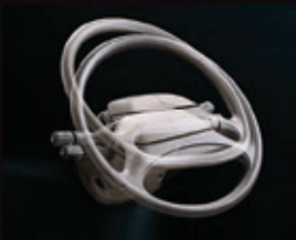
Protecting the driver Impact absorbing steering system
