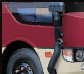
Snorkel air intake Protects engine from dust
