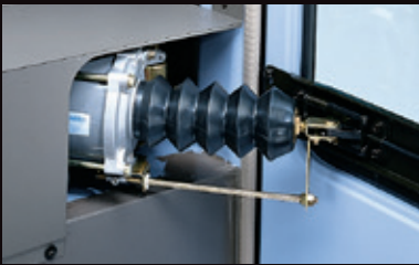
Adoption of a folding-type automatic door
