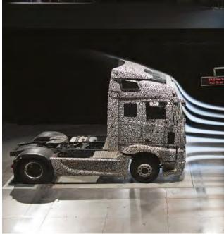
**Sophisticated aerodynamics.** When designing the new Actros we tested every individual part extensively – in the wind tunnel and on many million miles of test routes – for minimal drag and low fuel consumption.
