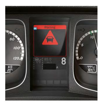
**Active Brake Assist 4**<sup>1).</sup> The fourth generation of the system assists the driver<sup>2) 3)</sup> by carrying out a full brake application in response to stationary and moving objects and partial braking in response to pedestrians in motion; in this way, it can reduce the severity of accidents or even prevent them completely.
