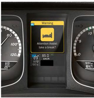
Attention Assist. Monitors the attention paid by the driver. It is based on the Lane Keeping Assist system. The attention paid by the driver is measured on the basis of the driver staying in-lane, in combination with various driver activities (direction indicator/accelerator/engine brake/retarder operation, etc.) as well as steering behaviour. The lane monitoring function continuously detects the position of the vehicle between the lane markings.
