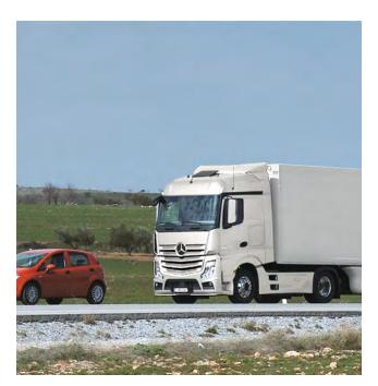
**Proximity Control Assist**<sup>1)</sup>. The safety system with stop-and-go function is on hand to support the driver in stressful situations and can reduce the risk of rearend collisions.
