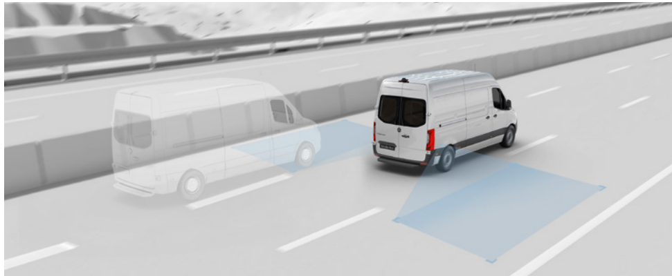
Blind Spot Assist with Rear Cross Traffic Alert can output visual and audible signals to help prevent accidents during lane changing, when reversing out of parking spaces and when alighting from the vehicle.
