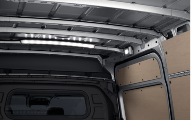
The two LED light strips under the roof illuminate the load compartment while largely avoiding shadows, for improved visibility inside when loading and unloading the vehicle.
