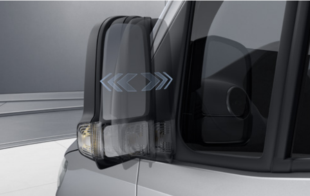
The electrically folding exterior mirrors are better protected against damage when folded in when space is tight in entrances and exits.
