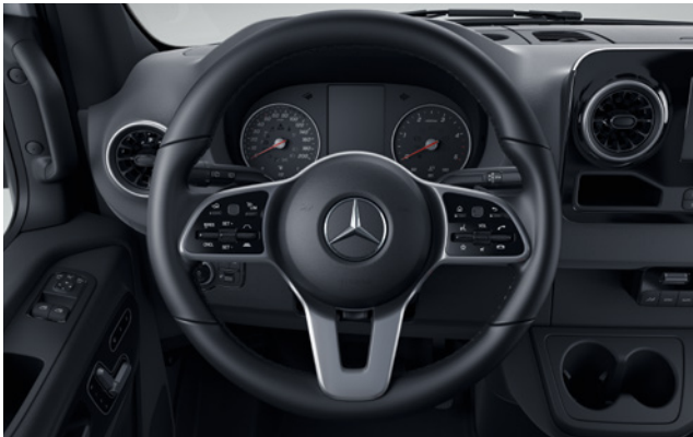
The multifunction steering wheel offers a convenient means of operating the on-board computer, vehicle functions and the multimedia systems via touch control or steering wheel buttons, without the driver having to remove their hands from the wheel.
