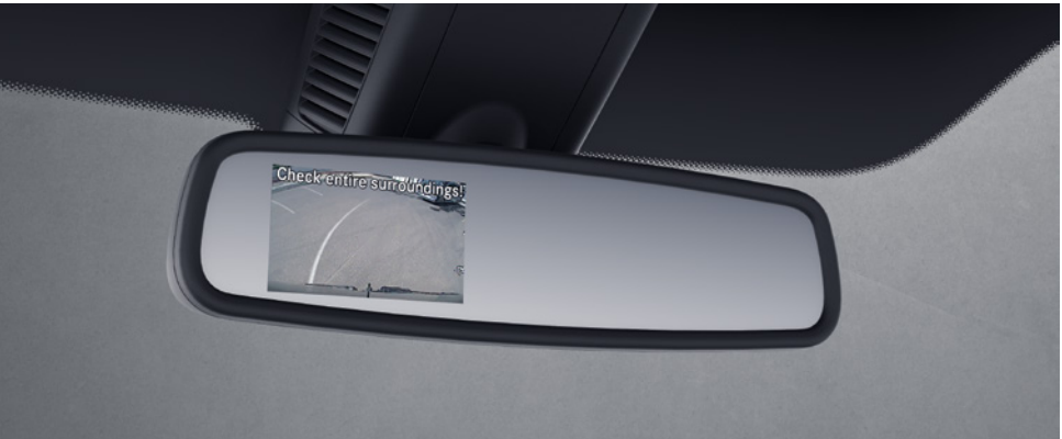
The reversing camera with rear-view mirror display improves the view of the area directly behind the vehicle and enhances safety when reversing.
