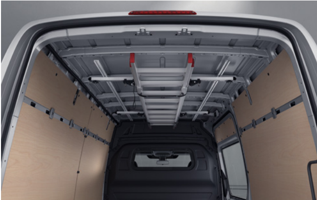
In comparison to externally fitted roof luggage racks, the roof luggage rack 1 in the load compartment offers transported items better protection from soiling and theft.
