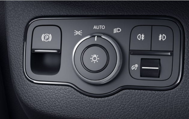
The electric parking brake is simply and conveniently operated via a button. It avoids the need for a parking brake lever, thereby facilitating access to the rear.
