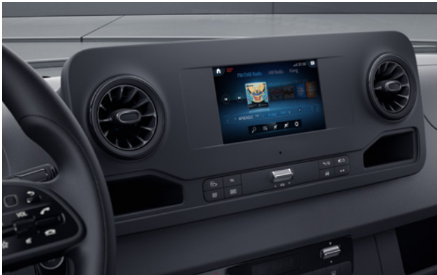
The MBUX multimedia system with 17.8 cm (7-inch) touchscreen boasts intuitive touch control, a high-resolution touchscreen and a wealth of communication and infotainment features.
