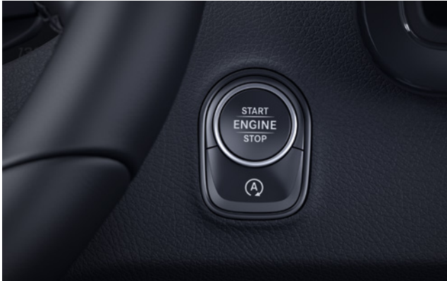
Starting the engine at the push of a button: the KEYLESS START drive authorisation system allows the engine to be started simply by pressing the start/stop button in the ignition lock.
