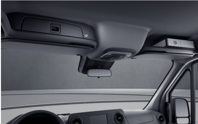
The conveniently accessible, lockable compartment on the left inside the compartment above the windscreen enables important items to be stowed away securely.
