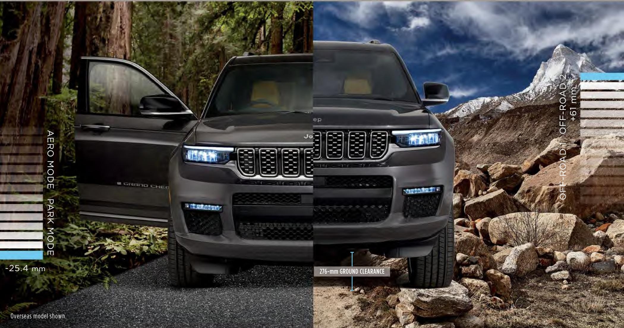
**QUADRA-LIFT® AIR SUSPENSION** This available system sets Jeep® Grand Cherokee L apart by lowering ride height for optimal access or rising higher to meet your on-road demands. Now, the system reacts even faster and raises even higher, so you're handed exceptional ground clearance with water fording<sup>2</sup> capabilities up to 610 millimetres.
